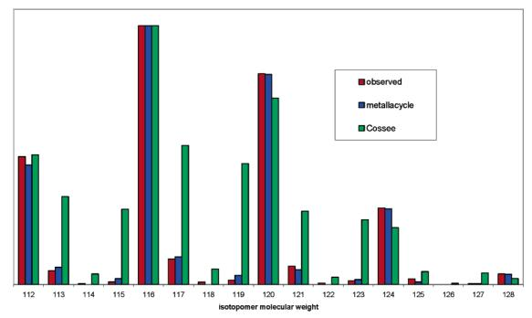
Figure 2. Observed 1-octene isotopomer distribution against predicted distributions for the metallacycle and Cossee-Arlman mechanisms.
