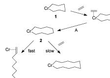
**Scheme 4.** Postulated Mechanisms for the Formation of Methylcyclopentane and Methylenecyclopentane
