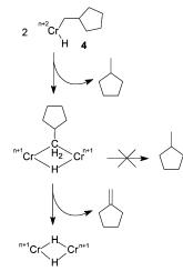
GC-MS analysis was made. This indicated the absence of the coupled product. Furthermore, tetramerisation reactions conducted in the presence of an excellent H• donor such as triphenylmethane still produce 1:1 ratios of the  $C_6$  cyclic products, where more methylcyclopentane may have been expected. These results strongly suggest that free radicals are not involved.
