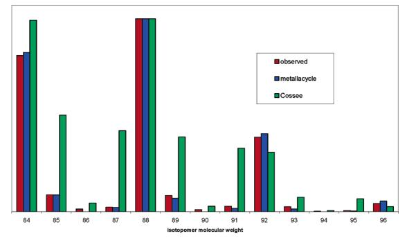
Figure 1. Observed 1-hexene isotopomer distribution against predicted distributions for the metallacycle and Cossee-Arlman mechanisms.
