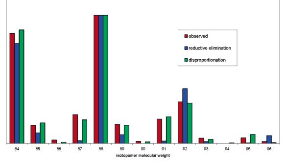
Figure 3. Observed methylcyclopentane isotopomer distribution against predicted distributions for the metal-mediated reductive elimination and dispropotionation mechanisms
